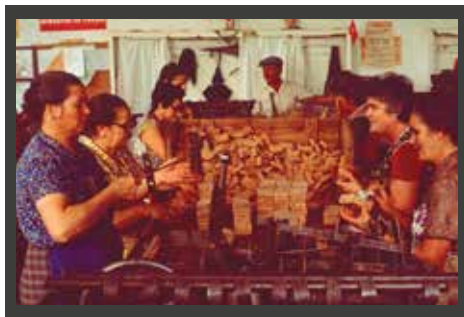
In some sections – for example, on the champagne stopper and cork paper production lines – manual (almost artisan) production coexisted with semi-automated processes.
